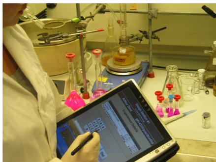
Figure 2. An example of a tablet PC as an interface onto the virtual electronic laboratory notebook (from the Smart Tea Group).
