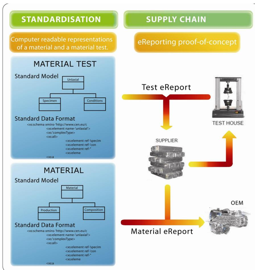
Figure 1. The use of standards for representing and reporting engineering materials data in the supply chain.
