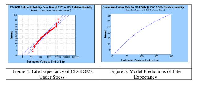
Applying the refined Ehring model enabled the prediction of end of life estimates for the CDs at different temperature and RH conditions. *Testing the Model.*
